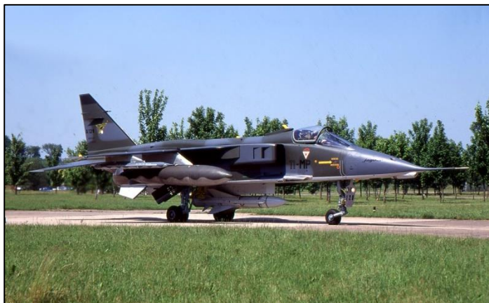
Le Jaguar A 129 en configuration missile anti radar, emportant un missile AS 37 Crédits P. Bigel.
